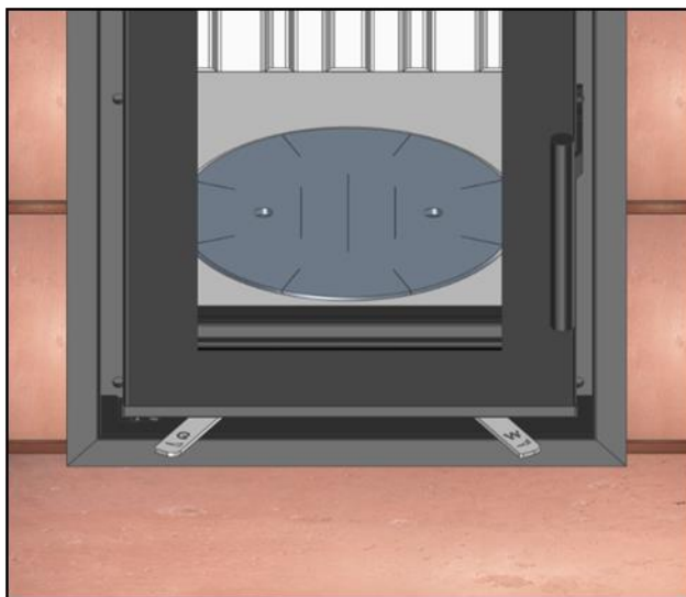
Fig.4 Setting regulators when choosing to burn wood logs
